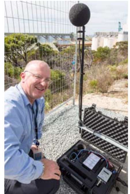
Environmental Manager Alex Leonard inspecting the new noise logger in Bostock Street
