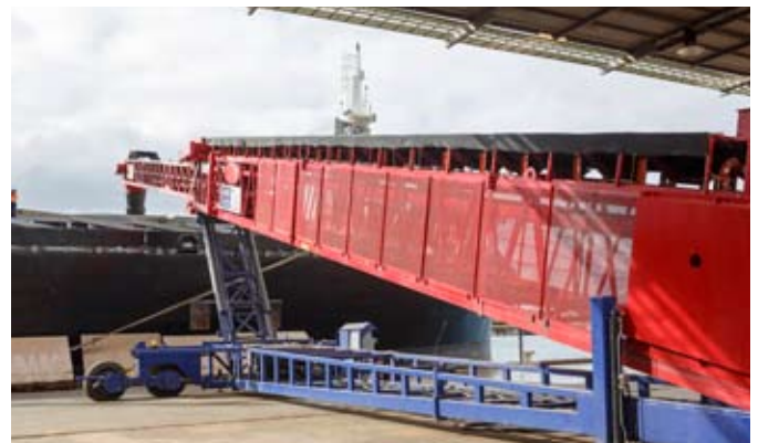
Mobile ship loading conveyor
