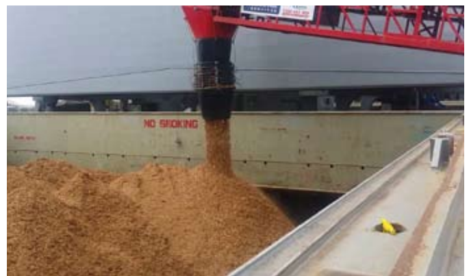
Woodchips conveyed by the mobile ship loader into the hull of the vessel
