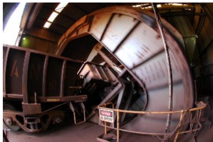
Above: Rotary car dumper in the process of unloading a wagon.
